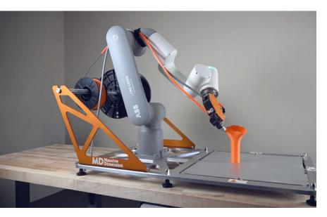
This 3D printing cell is a powerful solution that uses the ABB GoFa and Massive Dimension's filament extruder. This solution is ideal for colleges and universities as it includes comprehensive course materials and globally recognized STEM certification.
