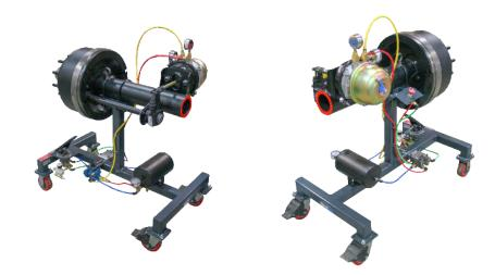
The ConsuLab HV-126-DM\_052960 trainer includes a heavy-duty trailer drum assembly with air chamber and wheel end. Using shop air (90 psi minimum) the service and parking brakes can be applied, the brake system can be dismantled, adjusted and the brakes can be measured. The trainer includes cutaways showing the s-cam, the slack adjuster and the bearing races.
