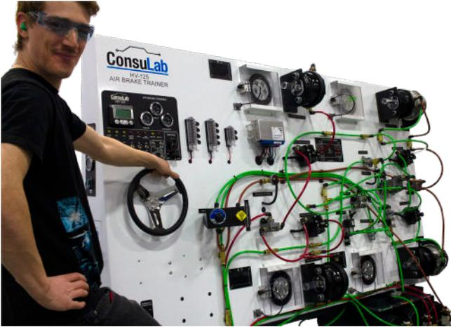
Meticulously designed as the premier air brake system training aid in the world. This product is comprised of a complete transit bus air brake system with all DOT approved components; disc brake systems, and all valving currently in use today. No legacy components here. This is the real deal.
