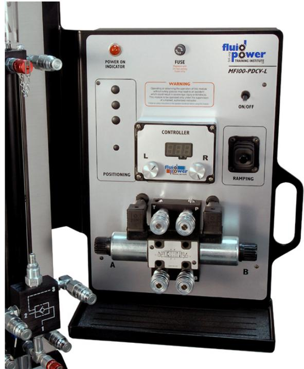
9. All hydraulic components are fitted with high-quality quick-connect/disconnect valves.
