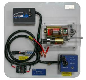
The EM-200-19 Starting System Trainer allows for the demonstration of a complete starting system using real-world components. Key areas of the starter have been cutaway to allow visual observation of major components while still being functional. Requires a 12V battery or jump box to operate.
