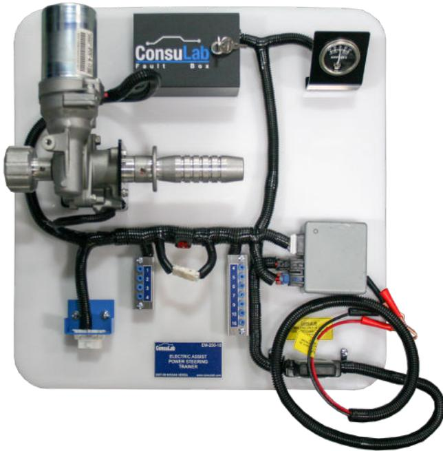
The ConsuLab EM-200-18 Electric assist power steering trainer is a functional column-mounted electric assist unit for use in a classroom environment. Once connected to a 12V battery and using the supplied handles, you and your students can vary the input torque with one hand and experience the output torque with the other hand all while viewing the scan tool data live through the provided OBD2 DLC and built-in ammeter.
