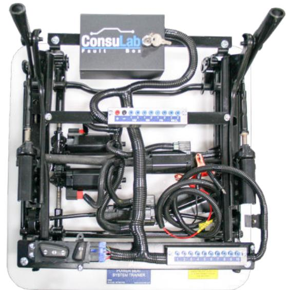
The EM-200-05 trainer allows for the demonstration of a complete power seat system using real-world components. Terminal block receptacles are provided for diagnostic test points.
