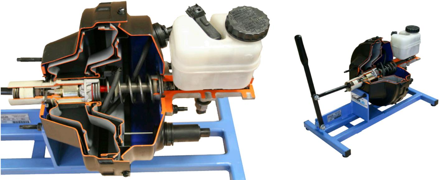
The ConsuLab EC-122 cutaway allows to visually demonstrate the operation and internal parts of a vacuum brake booster and master cylinder. The trainer is equipped with a braking handle that simulates the brake pedal for educational purposes. On a vehicle when the driver depresses the brake pedal, the movement is transformed into hydraulic pressure that is delivered to hydraulic cylinders at the four wheels through pipes and hoses using an incompressible fluid.
